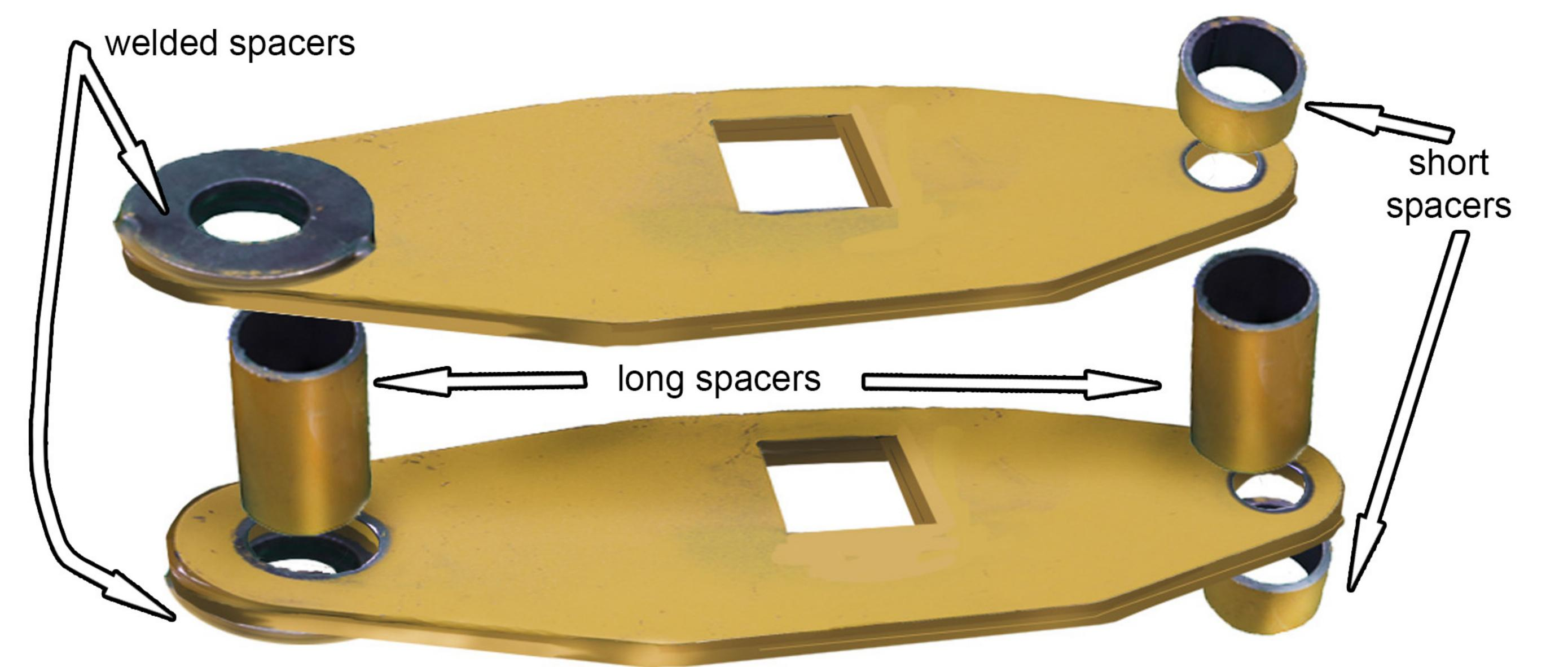
STEP 5 Lay center-link components into position. Identify the wider side of the attachment's keyways. Place the center-link square hole over the pivot block, welded spacers facing the narrow side. Set the spacers into position.
