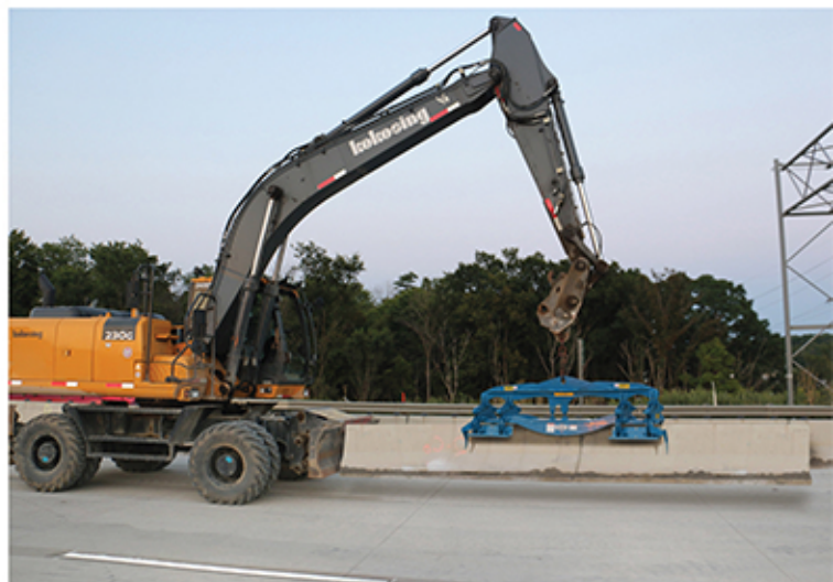
above: Kokosing Construction is seen using the Double Barrier Lift along Interstate 271 near Cleveland, Ohio.
