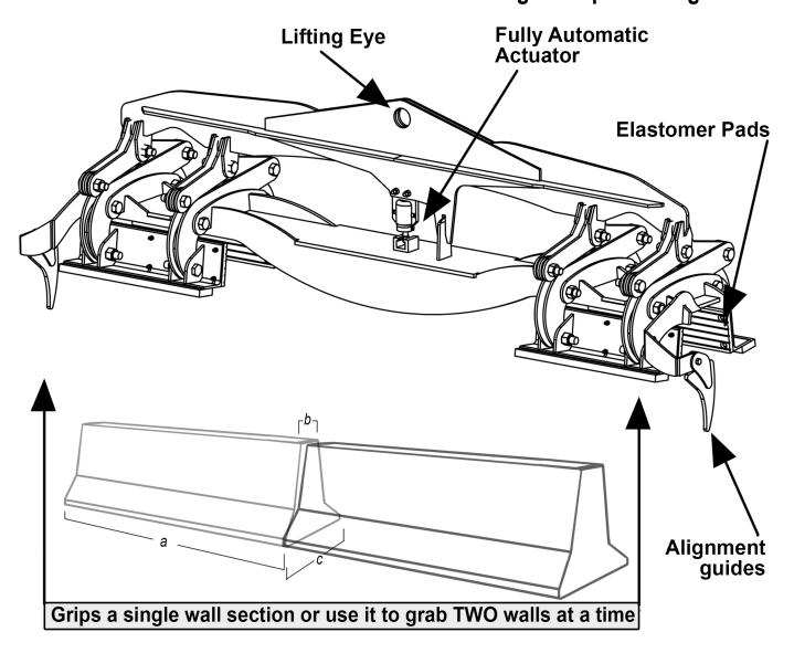
These lifting attachments are custom - built based on the (a) Length of wall \_\_\_\_ (b) Width of wall top \_\_\_\_ (c) Weight of wall
