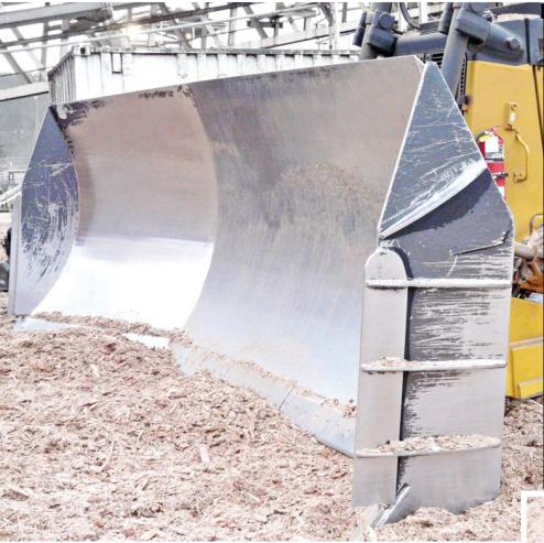
The Chip Blade is used primarily in the Pulp and Paper industry for the stockpiling of wood chips.
